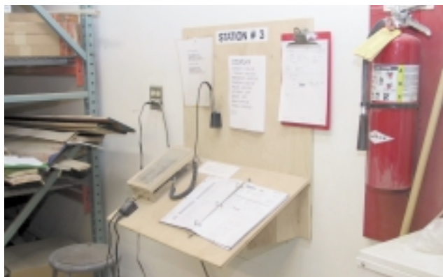
To use TradeSoft's ShopPak software, Masco Support Services installed bar code scanning stations called Tricoders for employees to track what they are working on.
